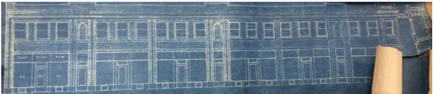
Figure 1: Architectural plan drawing of the south facade, created on January 1923 by the architecture firm of Charles Forrest. The drawing shows the intended tapestry-style brick veneer and Italianate projecting roof cornice, which are features of the finished building.
